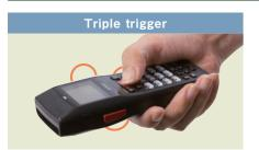
The triple trigger, which enables you to use both your thumb and index finger to scan, is adopted. You can scan barcodes and press keys without changing your grip
