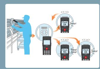
You can do 1:1 and 1:n matching using the first-read barcode as the master data for matching.
