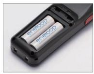
You can use "eneloop®" rechargeable batteries as the mainpower source The batteries are friendly to the environment as they can be used repeatedly and they also largely reduce the running costs per operation. Another benefit to using "eneloop®" rechargeable batteries is that unlike the special battery, they are easy to obtain. Of course, ordinary alkaline AA batteries may also be used.
