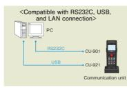
The terminal can communicate with devices in upper hierarchies through the communication unit.
