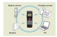
Bluetooth Ver. 2.1 is equipped. The terminal can communicate wirelessly with portable printers, PCs, Mobile phones, etc. Moreover using a Mobile phone, you can access the terminal through a modem. You can send data and request information such as stock data through it.
